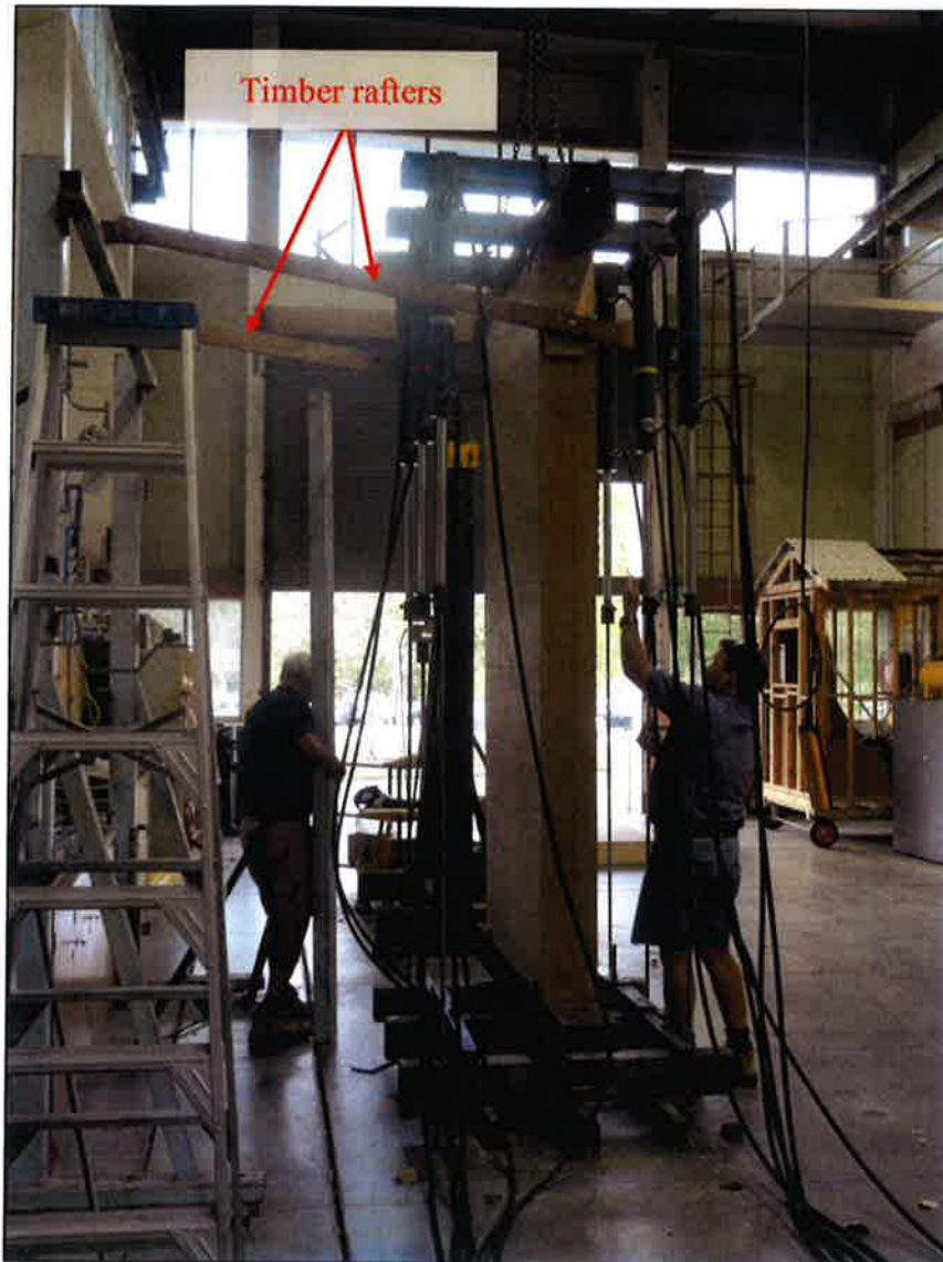
Figure 6: Sample Maintained in Vertical Position thanks to Timber Rafters
