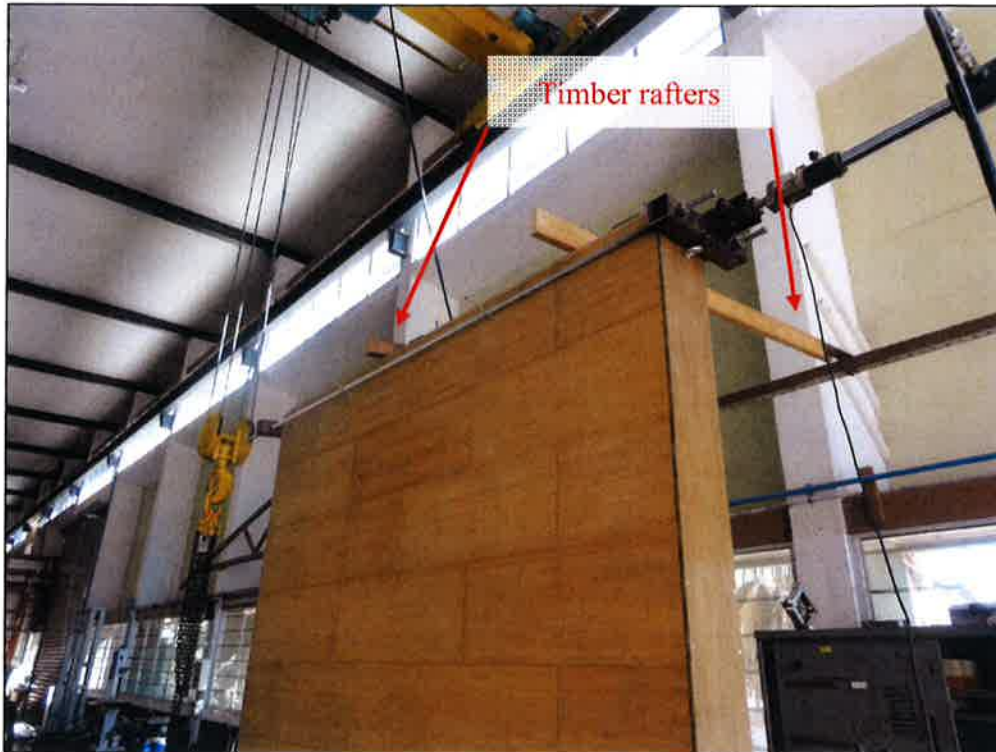
Figure 5: Sample Maintained in Vertical Position thanks to Timber Rafters
